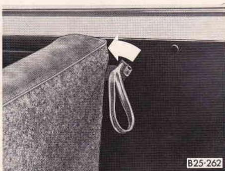
You can expand the luggage compartment load surface by folding the backrest of the rear seat bench down.
