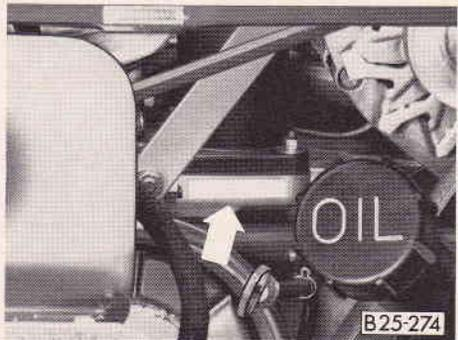
**The Engine Number (gasoline engine)** is located on the right side of the engine block.
