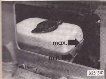
Refill tank Diesel engine
