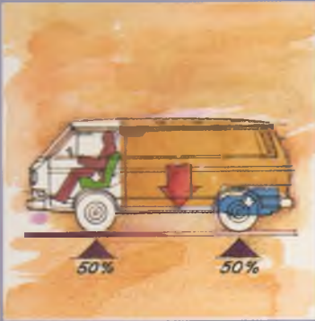
Vanagon's engine, transmission and final drive are located over the rear wheels for an optimum 50/50 weight distribution and increased directional control.
