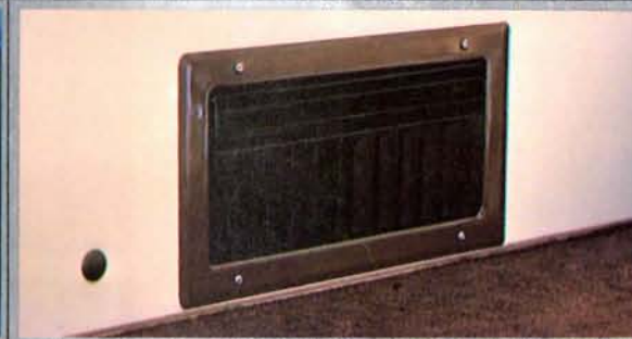
Blower-assisted rear heater outlets. (Left—Vanagon without trim panel; right—Vanagon Camper)
